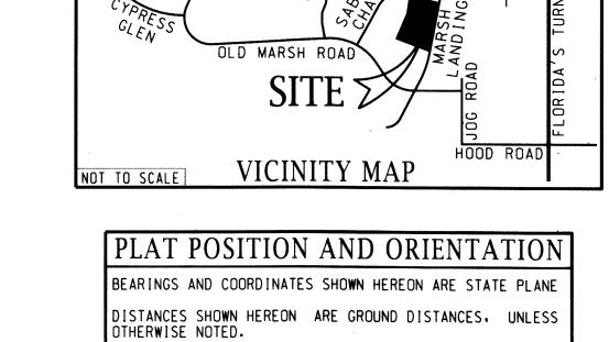
UNITS: US SURVEY FEET SCALE FACTOR: 1.000030297 GROUND DISTANCE X SCALE FACTOR = GRID DISTANCE PROJECTION: TRANSVERSE MERCATOR
